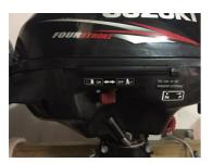
1) Check that the red lever is in the "ON" position
